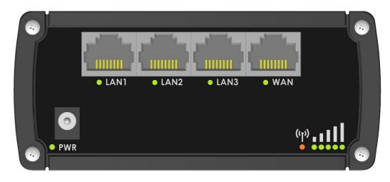
RUT9xx can be powered from power socket and over Ethernet simultaneously. Power socket has higher priority meaning that the device will draw power from power socket as long as it is available.
